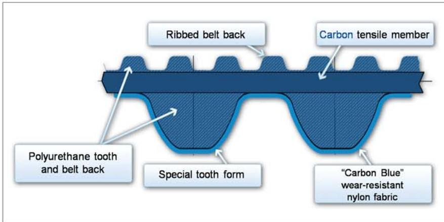
The surface of a synchronous belt is smooth, impervious, non-porous, non-absorbent and free of cracks and crevices, making it easily cleanable.
