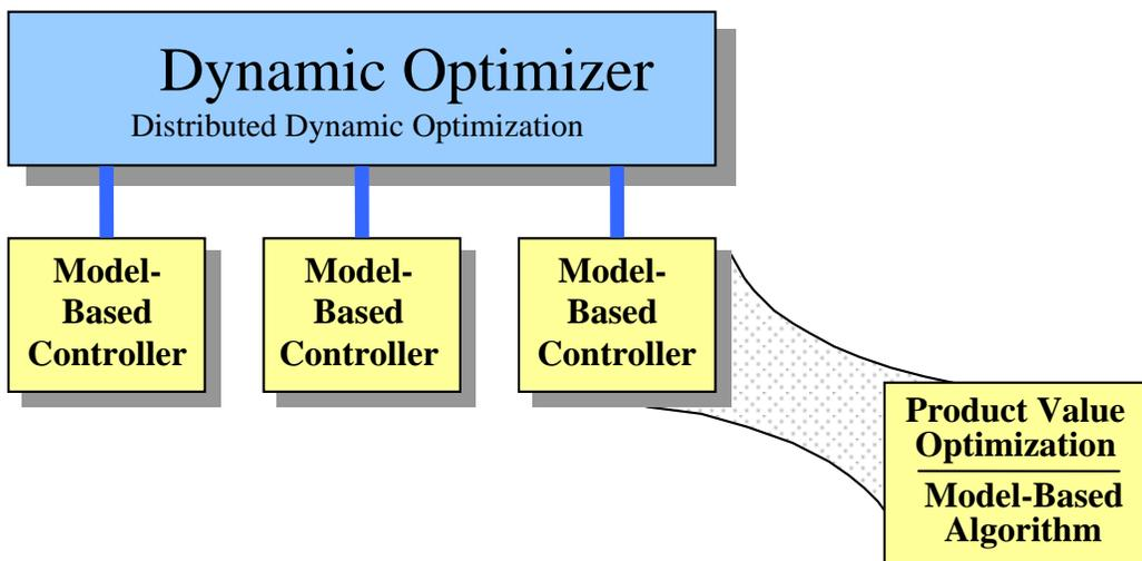
**Figure 6: Multiple unit optimization with dynamic optimizer**
