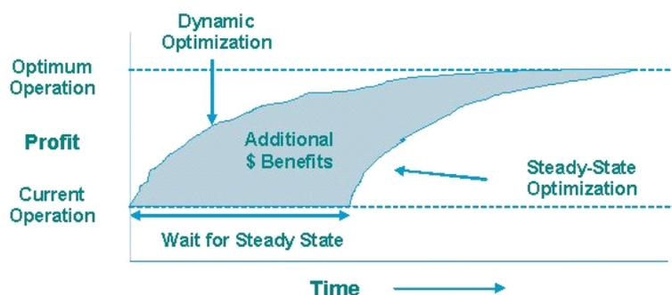
Figure 5: Comparison of dynamic and steady-state optimization
