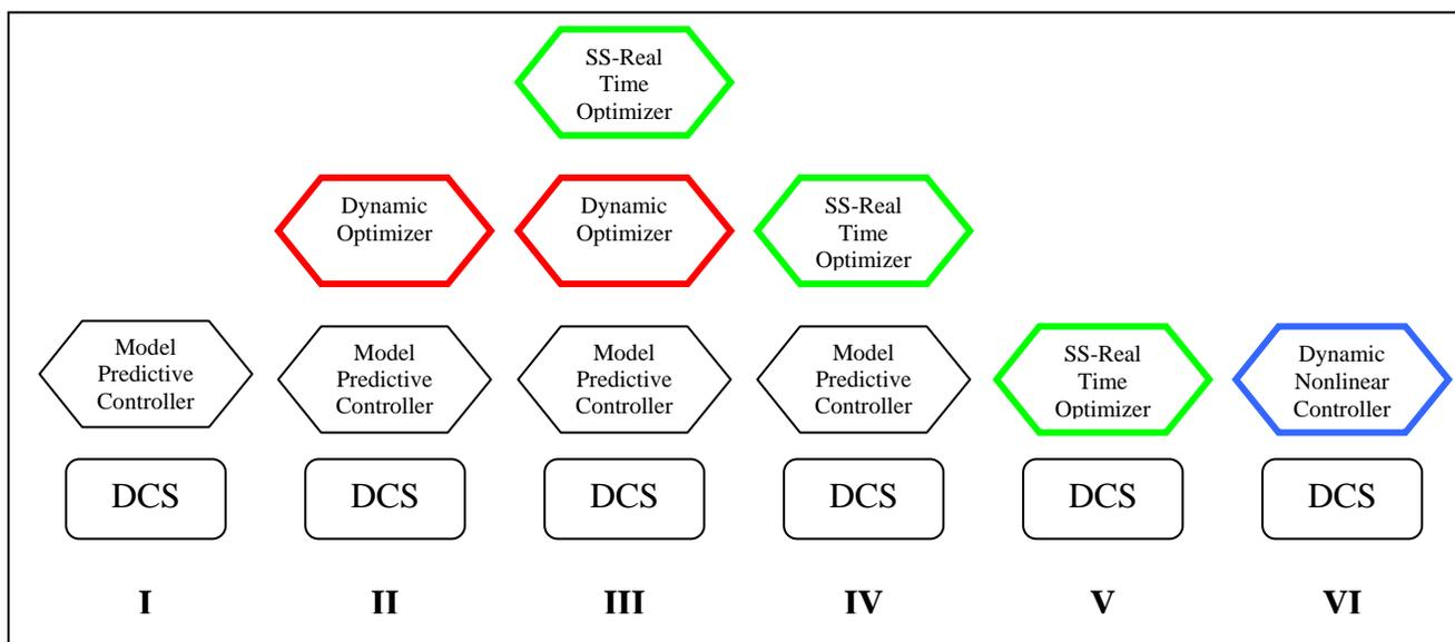
**Figure 2: Optimization Configurations**
