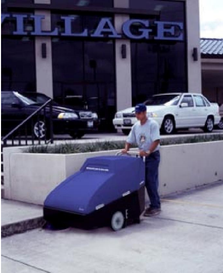
Battery powered walk-behind sweepers are suitable for indoor and outdoor areas not exceeding about 50,000 sq.
