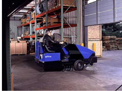
Mid-size sweepers are suitable for indoor and outdoor surfaces up to 130,000 sq. ft.
