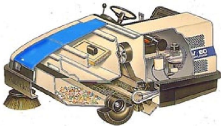
ft. Cutaway shows the “dustpan” design of this mid-size 60” ride-on sweeper.
