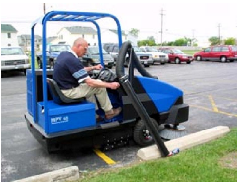
Accessories such as this vacuum wand assist in picking up large debris out of the roadway.
