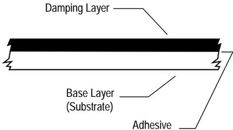
Figure 6: Extensional (Free-layer) Damping Construction, Cross Section
