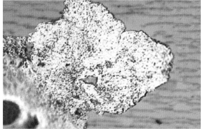
*White metal particle misaligned with magnetic field*
