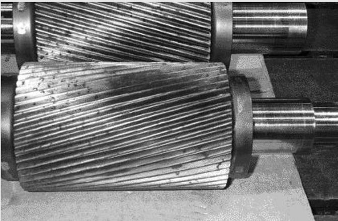
*Lubrication failure led to severe damage to the gearbox (above)*
