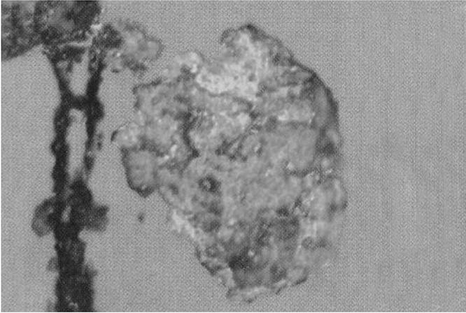
Sample of magnified oil analysis indicating roller contact failure
