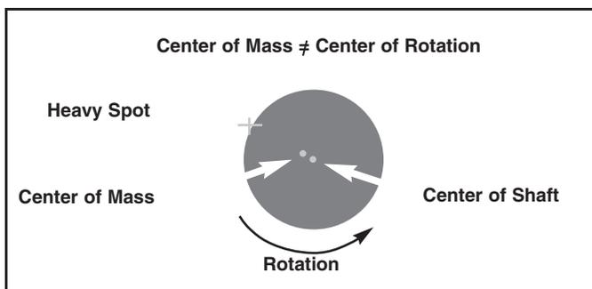
Imbalance can cause other gear faults to appear
