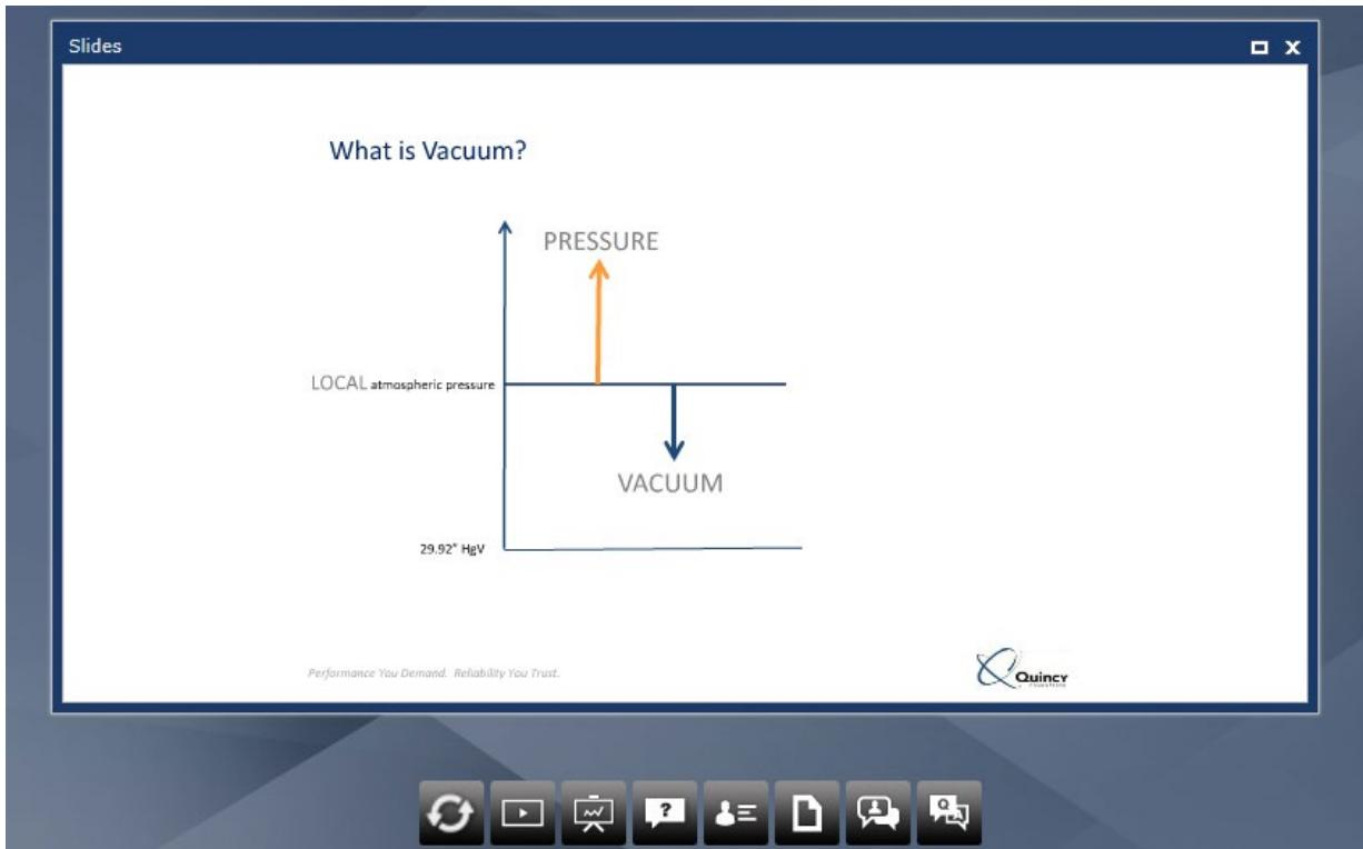
example, a vane vacuum that can get down to 29.9”HgV does not mean that all vane vacuums can get to 29.9”HgV or cannot go lower; it just means that that is the specific design of that unit.”
