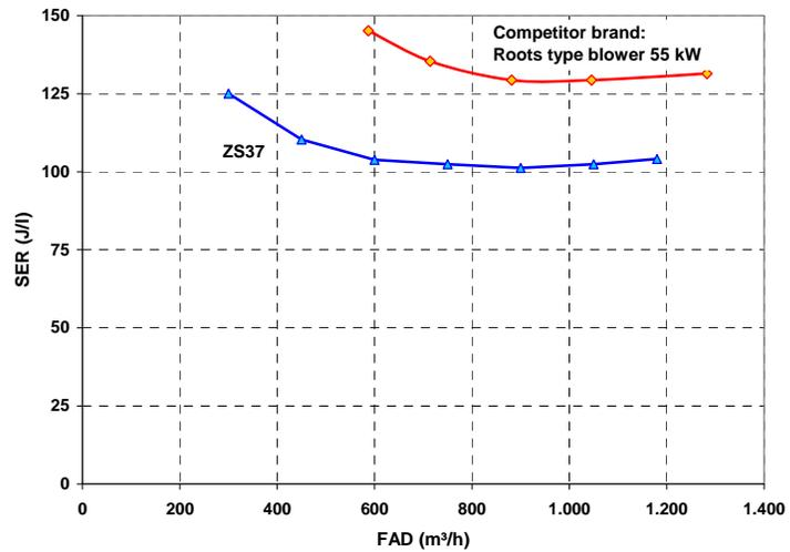
In addition to these tests it was determined that an independent audit to witness the testing of a screw blower against a tri-lobe blower may bring an objectivity otherwise not available . The below certificate shows the results of the independent performance test.
