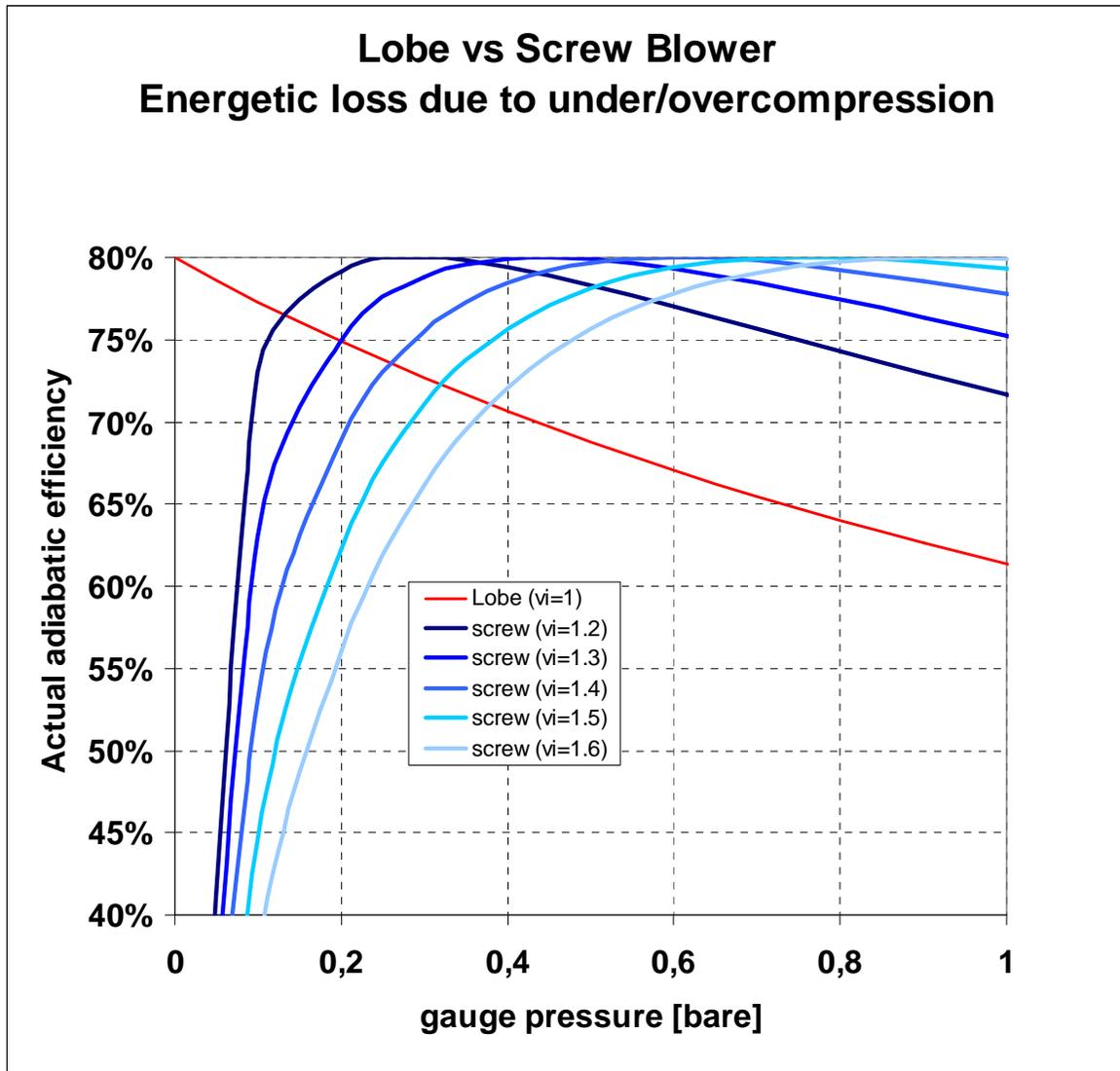
figure 8 : actual adiabatic efficiency screw vs lobe
