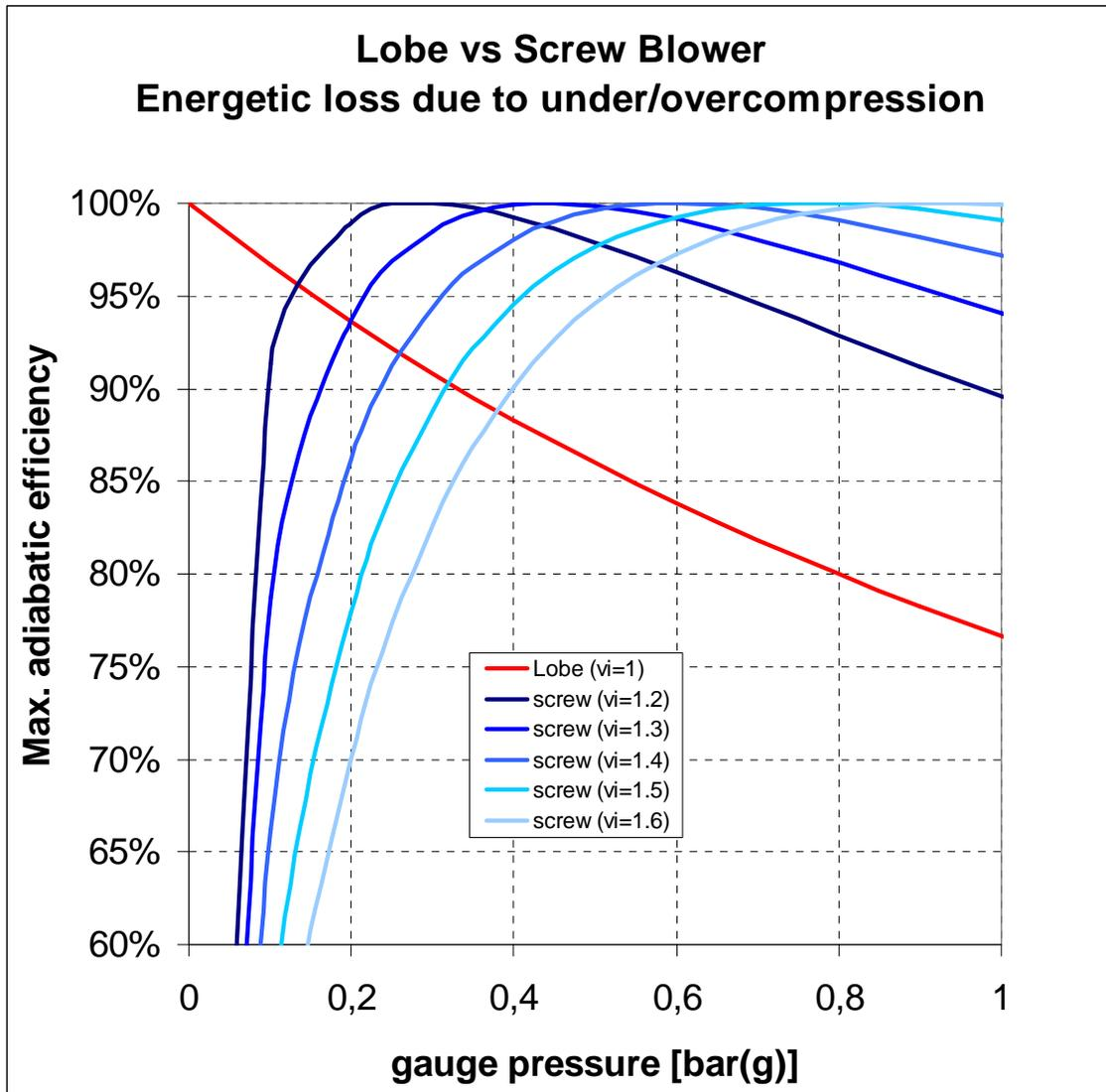
figure 7: maximum adiabatic efficiency screw vs lobe
