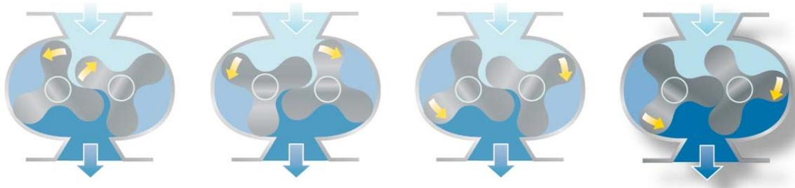
figure 1: working principle of a lobe type blower
