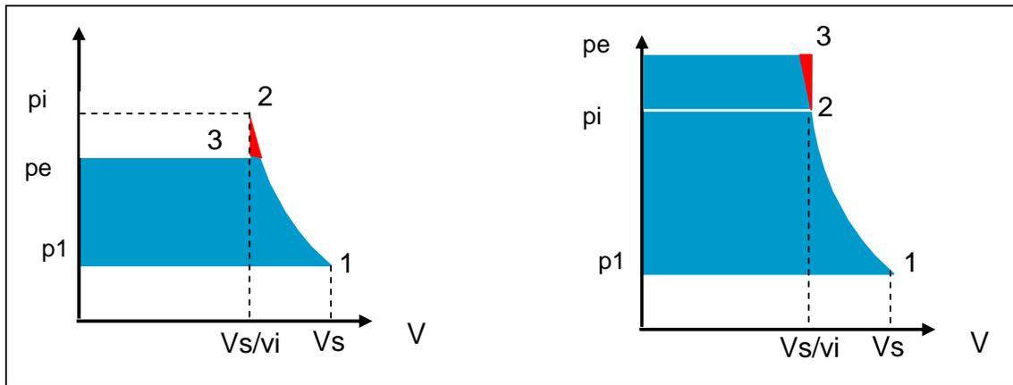
figure 6 : over compression (left); under compression (right)
