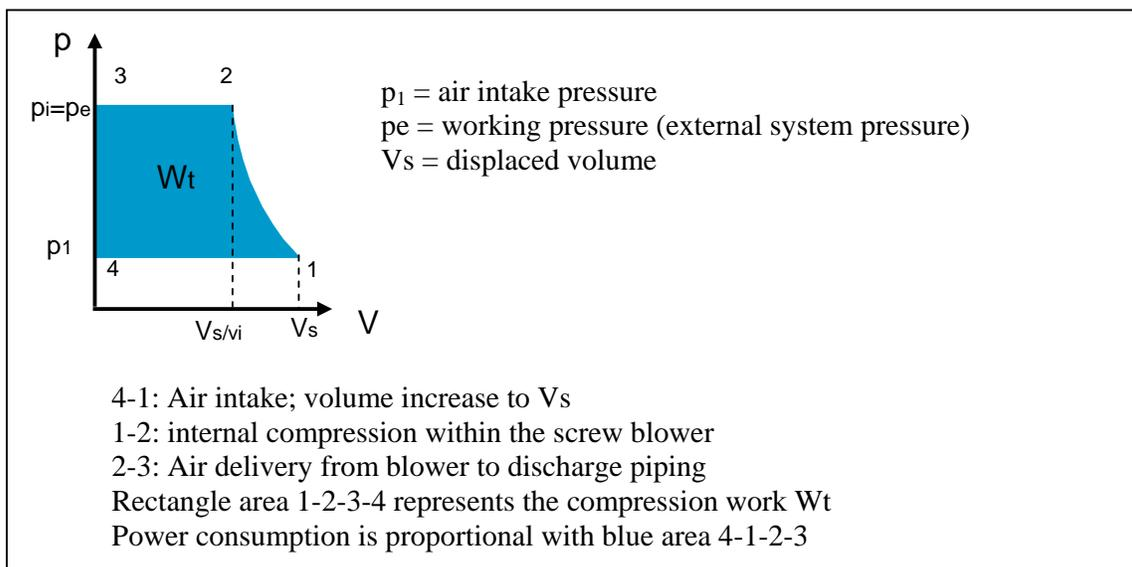
figure 4 :  $pV$  diagram screw blower with  $p_i = p_e$
