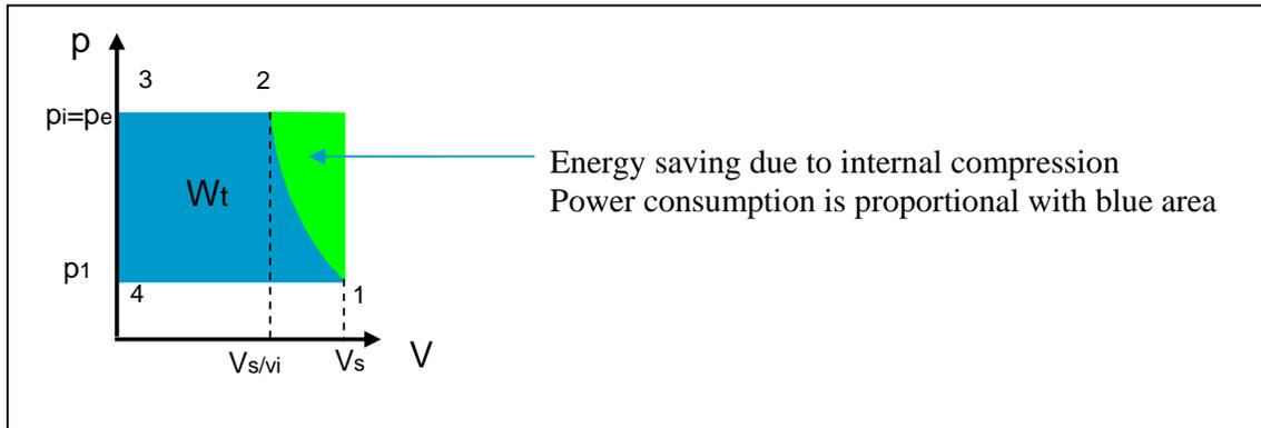
figure 5 : Energy saving screw blower vs lobe blower
