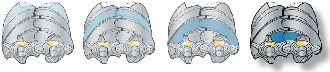
figure 2 : working principle screw blower
