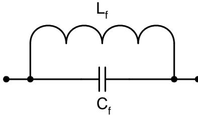
**Fig. 2.** Single-phase representation of a series filter configuration.
