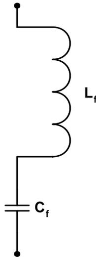
**Fig. 3.** Single-phase representation of a shunt-tuned filter configuration.
