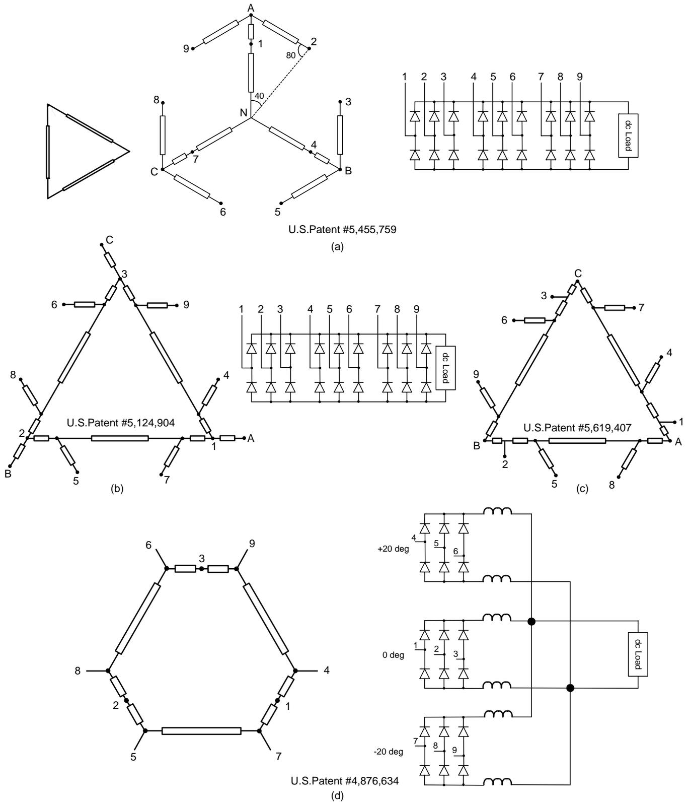
**Fig. 11.** Autotransformer methods of achieving 18-pulse operation.
