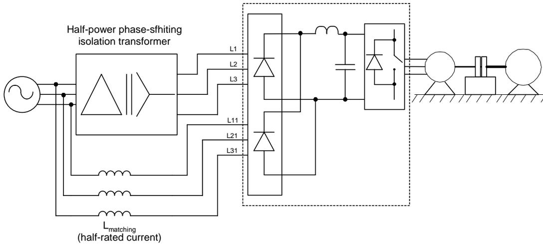
**Fig. 7.** Schematic of a pseudo 12-pulse arrangement.
