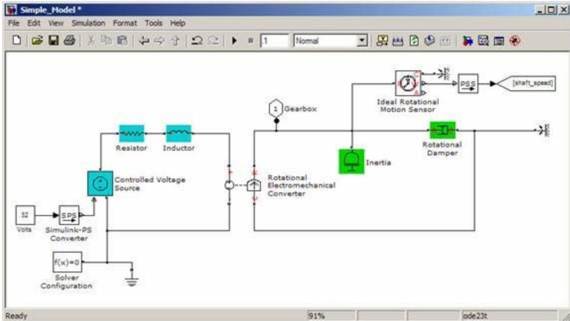
**Figure 3. A model of a DC motor developed using physical modeling. Blocks highlighted in blue represent electrical components; blocks highlighted in green mechanical components**
