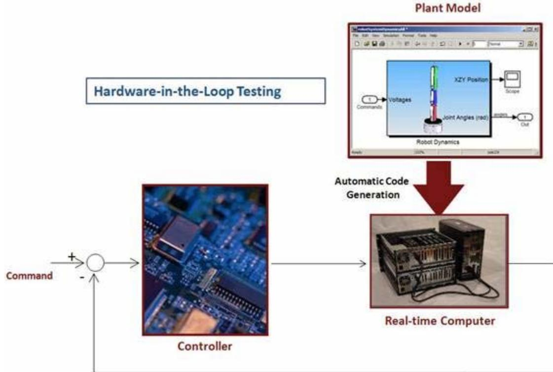
**Figure 1. Using the plant model for real-time testing of control algorithm (hardware-in-the-loop testing)**
