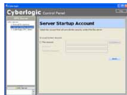
Image 5: Cyberlogic Crosslink executes as a Windows Service. Crosslink’s configuration enables users to bypass DCOMCNFG to set the Server’s execution either as System, or a specific User Account.
