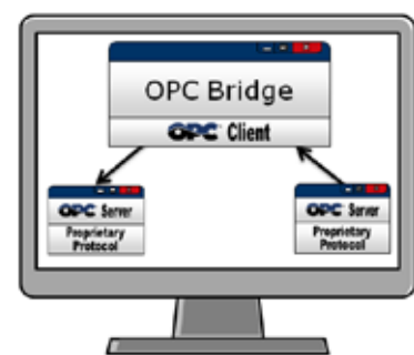
Image 2: The only way for two OPC Servers to communicate is to have an OPC Client application provide a bridge between the two servers, thus becoming an “OPC Bridge.”
